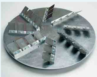
Bladed disc with metal or plastic blades for planing (filling in surface irregularities) magnesite screed
