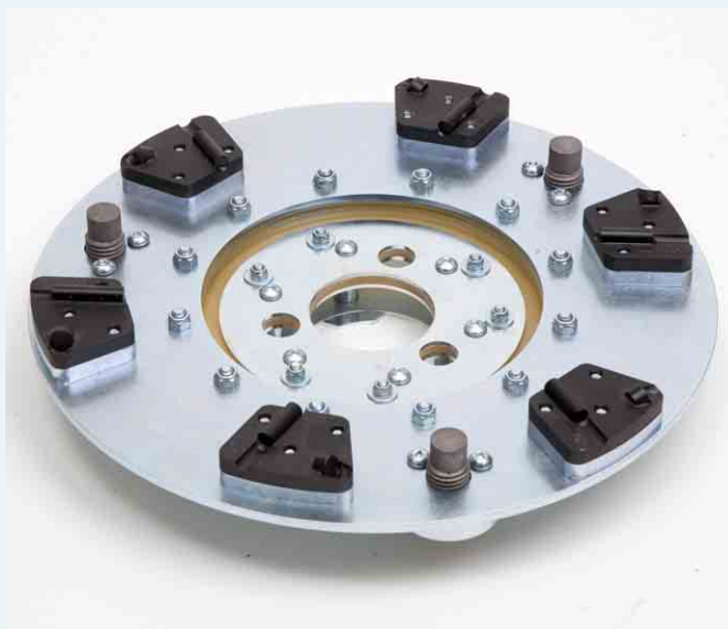
Drive plate PCD, buffered, Ø 400 mm with 6 PCD segments DFS-1 (black) and control of cutting depth. For the removal of stubborn adhesives (PU, bitumen, synthetic resin, etc.) and filler. Also for abrading screed, tile adhesive. Extremely efficient with a long tool life.
