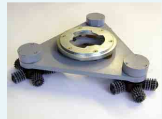
Drive plate WCT, buffered, Ø 425 mm, with 3 rotating cutting heads, WCT spiked - 2.5 mm for thin adhesives, paints, also on wooden floors. Or WCT spiked - 4 mm for adhesives, filler on very soft screeds.
